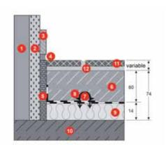
1 Wall 2 Coating 3 Skirting board 4 Elastic jointing material 5 FV THERM edge insulation 6 Seamless flooring as per DIN 18560 7 FV THERM system heating pipe PE-RT 15 mm 8 FV THERM staple 9 FV THERM system layered sheet PUR 14 mm 10 Backing 11 Tiles
