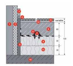
1 Wall 2 Coating 3 Skirting board 4 Elastic jointing material 5 FV THERM edge insulation 6 Seamless flooring as per DIN 18560 7 FV THERM system heating pipe PE-RT 15 mm 8 FV THERM staple 9 FV THERM EPS tacker roll 30 mm 10 Backing 11 Tiles 12 Thin-film elastic construction adhesive 13 EPS 30 mm sheet
